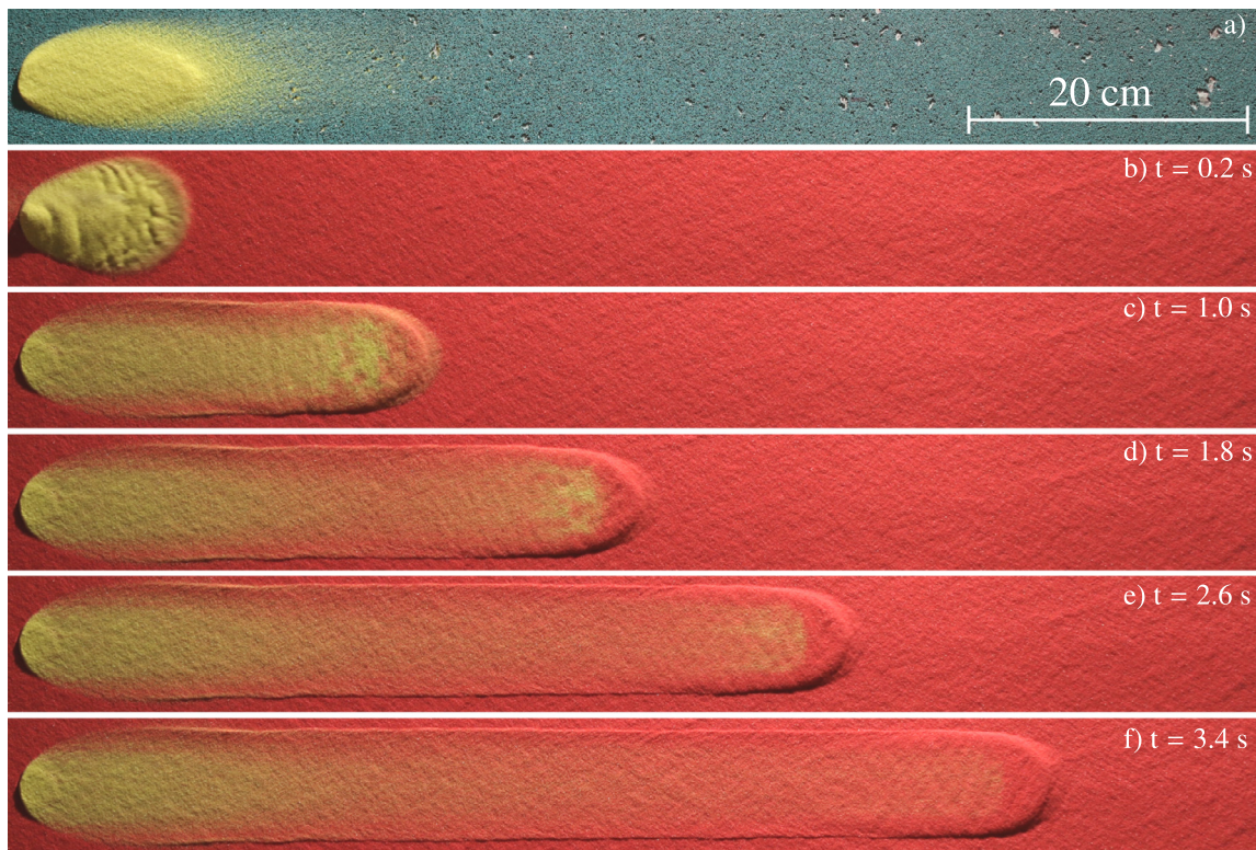
Fig. 3. Propagation of a single avalanche on a 34.0^\circ slope. a) Deposit without an erodible layer. b)–f) Steady travelling wave propagating on an erodible layer of thickness h_{stop}(34.0^\circ) \approx 1.7 mm. All of the initially released yellow sand is deposited during the flow, resulting in a steady avalanche that is composed entirely of red particles eroded from the bed. The same configuration is shown in movie 1 in the online supplementary material.
