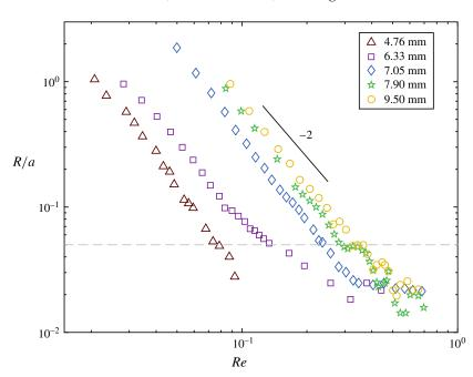
FIGURE 7. (Colour online) Non-dimensional orbit radius R/a, plotted against Re. The grey dashed line denotes the threshold below which a sphere is assumed to lie on its equilibrium point.
