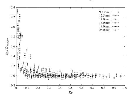
FIGURE 9. Graph of the frequency of oscillation of spheres in the diameter range 9.5–25.0 mm plotted as a function of *Re*. The frequencies have been made dimensionless using the rotation frequency of the cylinder.
