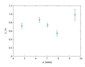
FIGURE 5. (Colour online) Non-dimensional horizontal displacement of the sphere at the onset of instability,  $x_c/a$ , as a function of sphere radius a.
