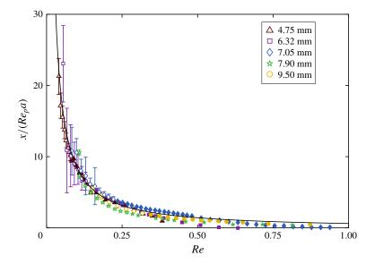
FIGURE 4. (Colour online) Horizontal displacement of the sphere as a function of Reynolds number for spheres of radii a = 9.5, 7.9, 7.05, 6.33, 4.78 mm. Open circles denote the centre of an orbit; filled circles indicate stationary fixed points. Each data point corresponds to the distance between the central axis of the cylinder and the centre of the sphere, averaged over 2 s (60 frames). The continuous line is the theoretical prediction for this horizontal displacement, from § 2.
