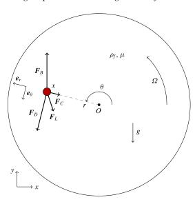
FIGURE 1. (Colour online) Schematic of an end view of the flow domain. A cylinder of fluid (outer circle) rotates about its axis O at angular velocity  $\Omega$ , and a buoyant particle of radius a (inner filled circle) is held at an equilibrium position by a balance of Stokes drag  $F_D$ , centripetal forces  $F_C$ , buoyancy  $F_B$  and lift  $F_L$ .
