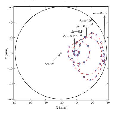
FIGURE 8. (Colour online) Plot of the orbits of a 12.5 mm sphere at the various given values of Re, illustrating the behaviour of the orbits as they approach the side wall of the drum (solid black circle).
