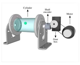
FIGURE 2. (Colour online) Schematic diagram of the experiment. A glass cylinder was mounted horizontally between bearings and completely filled with glycerol. A light sphere was placed inside it and the cylinder was rotated around its axis using a motor, a gear box and a smooth belt. A shaft encoder was used to measure the frequency of rotation of the cylinder.
