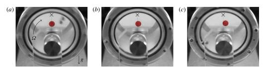
FIGURE 3. (Colour online) Sphere of radius a = 7.90 mm (false-colour shaded red, online) at different Reynolds numbers. The rotational axis of the drum is marked by a dotted line and a cross where this axis meets the far wall of the drum. As Re decreases, the horizontal displacement of sphere equilibrium position from this axis, x, moves further from the cylinder axis. (a) Re = 1.990,  $x \approx 0$  mm; (b) Re = 0.792, x = 1.8 mm; (c) Re = 0.7920.332, x = 6.25 mm.
